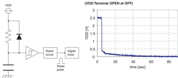
When the power is turned on, the power-on reset should be activated. If the power-on reset is not working properly, it can be returned to normal operation by executing reset using the asynchronous reset pin, hardware reset or software reset.
