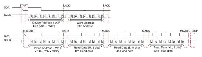
Pressure/Temperature data consists of 24 bits and output as three blocks of 8 bits. Data will be output as H, L and XL order and each 8 bits also output as MSB first.
