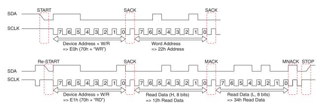
Set VBGACT bit "L" of I2C\_AADJ before this operation. Each 8 bits data will be output as MSB first.
