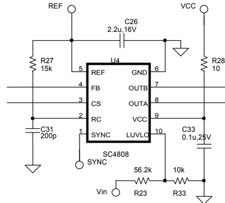
The oscillator has a ramp voltage of about Vref/2. The oscillator frequency is twice the frequency of the OUTA and OUTB gate drive controls.
