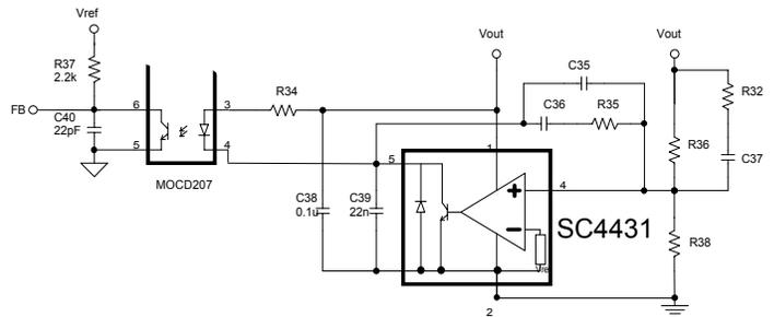
The signal at the FB pin is then compared to the 3X amplified signal from the current sense/ slope compensation CS pin. Matched out of phase signals are generated to control the OUTA and OUTB gate drives of the two phases. A single ramp signal is used to generate the control signals for both phases, hence achieving a tightly matched per phase operation.
