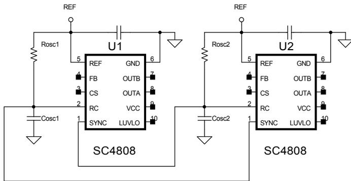
In the Bi-phase operation mode a very unique oscillator is utilized to allow two SC4808C's to be synchronized together and work out of phase. This feature is set up by a simple connection of the SYNC input to the RC pin of the other part. The fastest oscillator automatically becomes the master, forcing the two PWMs to operate out of phase. This feature minimizes the input and output ripples, and reduces stress on the capacitors.
