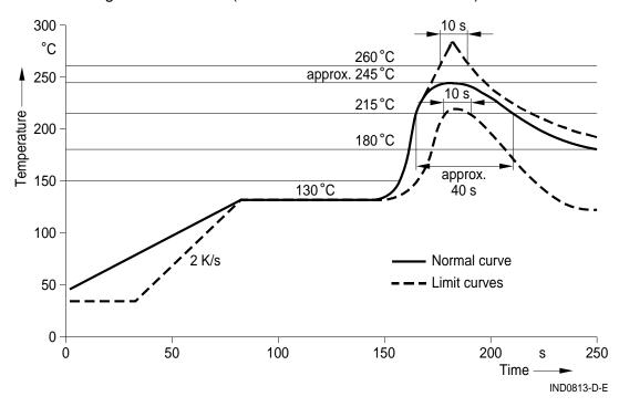
Pb-free solder material (based on JEDEC J-STD 020C)
