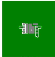
b. 55 °C/W when mounted on a 1 in<sup>2</sup> pad of 2 oz copper
