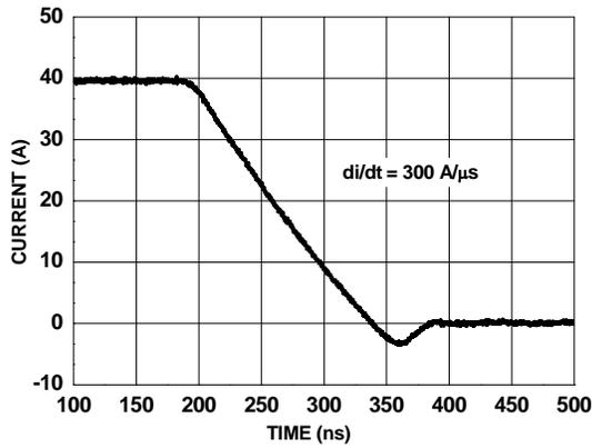
Figure 27. FDPC8014AS SyncFET™ Body Diode Reverse Recovery Characteristic
