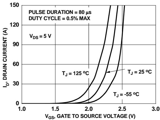
Figure 18. Transfer Characteristics
