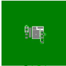
a. 60 °C/W when mounted on a 1 in<sup>2</sup> pad of 2 oz copper
