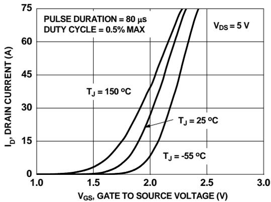
Figure 5. Transfer Characteristics
