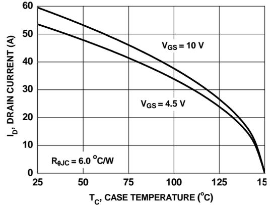
**Figure 10. Maximum Continuous Drain Current vs. Case Temperature**
