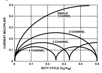
FIGURE 13. CURRENT MULTIPLIER vs DUTY CYCLE
