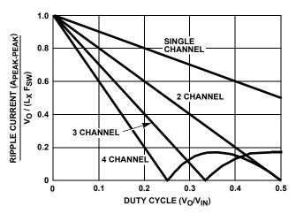
FIGURE 12. RIPPLE CURRENT vs DUTY CYCLE
