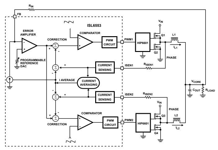
FIGURE 1. SIMPLIFIED BLOCK DIAGRAM OF THE ISL6553 VOLTAGE AND CURRENT CONTROL LOOPS FOR A TWO POWER CHANNEL REGULATOR
