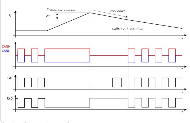
Figure 8 Overtemperature protection
