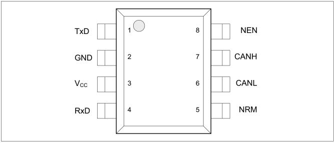
Figure 2 Pin configuration
