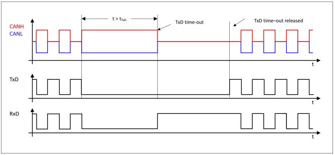
Figure 7 TxD time-out function
