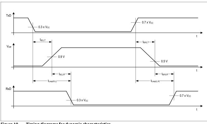
Figure 10 Timing diagrams for dynamic characteristics
