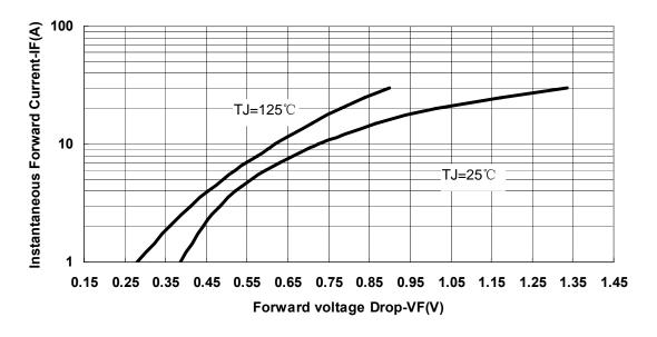
Fig.3-Typical Instantaneous Forward Voltage Characteristics
