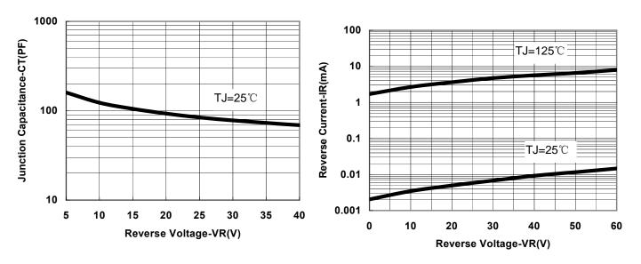
Fig.1-Typical Junction Capacitance
