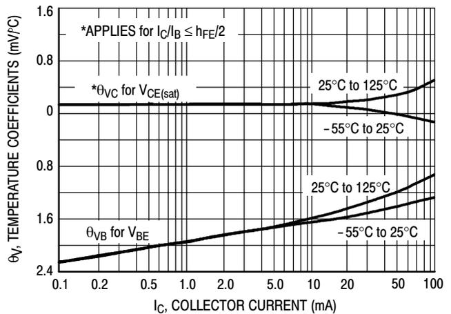
Figure 10. Temperature Coefficients
