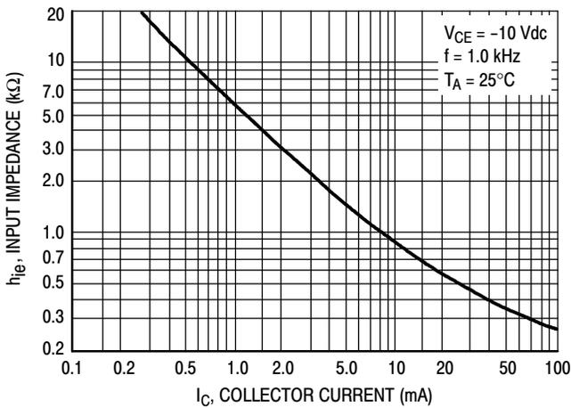
Figure 15. Input Impedance
