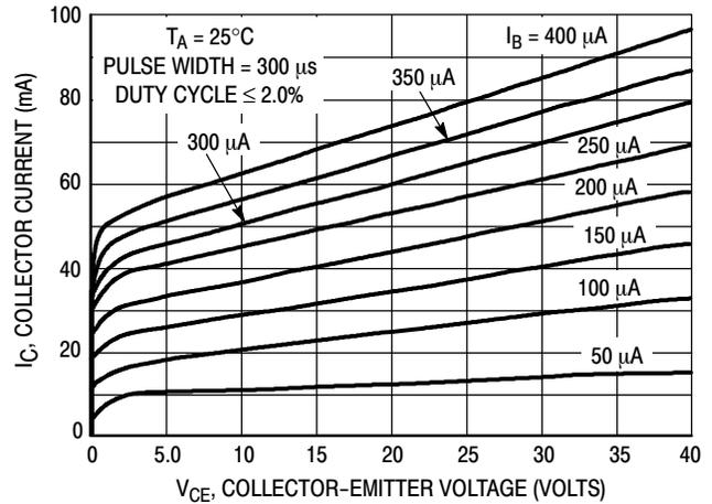
Figure 8. Collector Characteristics
