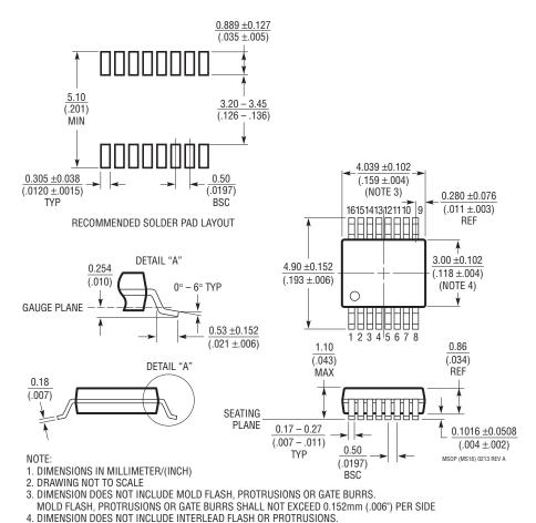
INTERLEAD FLASH OR PROTRUSIONS SHALL NOT EXCEED 0.152mm (.006") PER SIDE 5. LEAD COPLANARITY (BOTTOM OF LEADS AFTER FORMING) SHALL BE 0.102mm (.004") MAX
