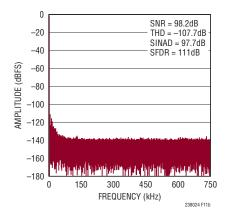
Figure 11a. LTC6362 Configured to Accept a ±3.28V Input Signal While Running from a Single 5V Supply When Digital Gain Compression Is Enabled in the LTC2380-24
