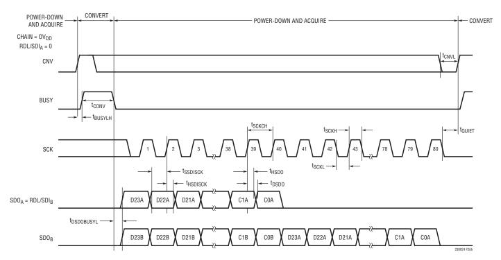
Figure 25. Chain Mode Timing Diagram
