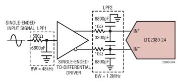
Figure 4. Input Signal Chain
