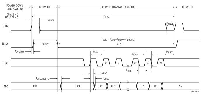
Figure 23. Using a Single LTC2380-24 in Normal Mode
