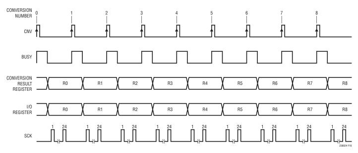
Figure 16. Conventional SAR Operation Timing
