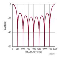
Figure 21. SINC<sup>1</sup> Filter with  $f_{SMPL} = 2Msps$  and N = 8
