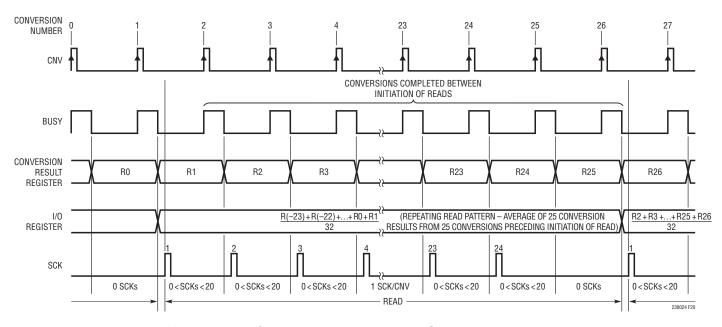
Figure 20. Averaging 25 Conversion Results and Reading Out Data with a Distributed Read
