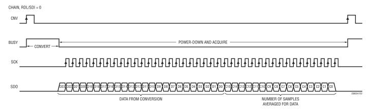
Figure 22. Serial Output Code Parsing
