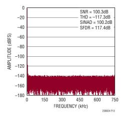
Figure 13. 128k Point FFT Plot of the LTC2380-24 with  $f_{IN}$  = 2kHz and  $f_{SMPL}$  = 1.5MHz
