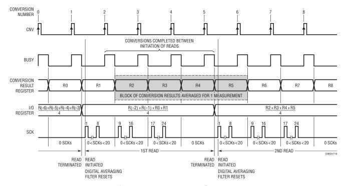
Figure 19. Averaging 4 Conversion Results and Reading Out Data with a Distributed Read
