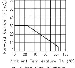
Fig. 3 FORWARD CURRENT DERATING CURVE
