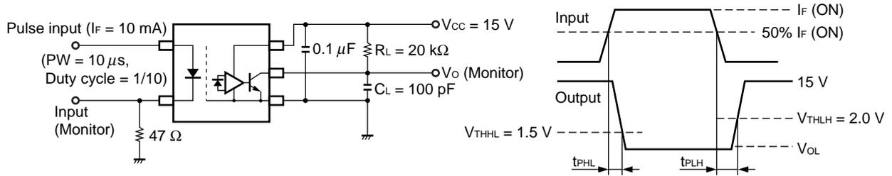
$C_L$  includes probe and stray wiring capacitance.
