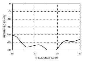
Note: Measured Performance Characteristics (Typical Performance at 25°C) Vdd1 = Vdd2 = 4.5 V, Idd1 + Idd2 = 400 mA
