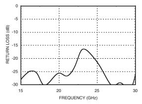
**Output Return Loss vs. Frequency**
