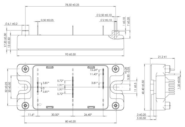
ALL DIMENSIONS MARKED "\*" ARE TOLERANCED AS : [  $\phi$  |  $\phi$  | 1
