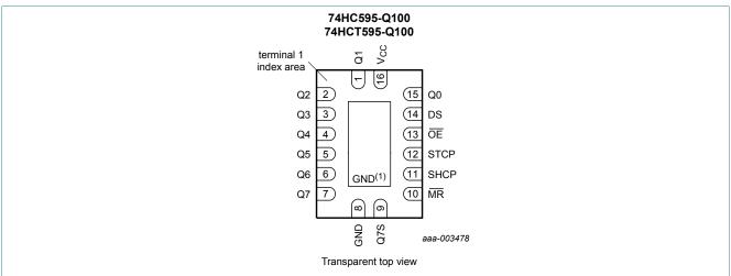
(1) This is not a supply pin. The substrate is attached to this pad using conductive die attach material. There is no electrical or mechanical requirement to solder this pad. However, if it is soldered, the solder land should remain floating or be connected to GND.
