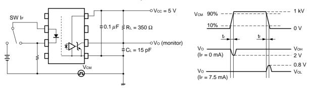
Remark CL includes probe and stray wiring capacitance.
