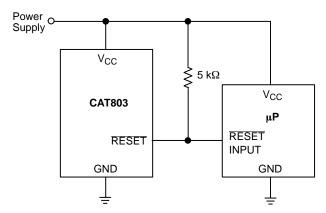
Figure 11. Typical CAT803 Open-Drain Circuit Configuration
