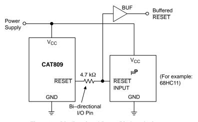
Figure 10. Bi-directional Reset Pin Interfacing
