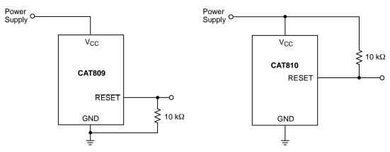
Figure 8. RESET Valid with V<sub>CC</sub> Under 1.0 V
