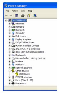
The "USB Device" can be opened to view it's uninstalled properties.
