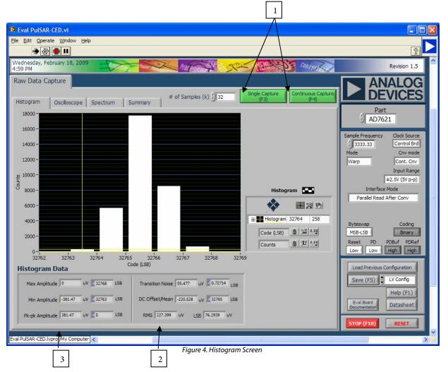
**1.** These radio buttons are used to perform a Single Capture or Continuous Capture of data set in the # of Samples field. The results are displayed in the chart. Note that the results can be displayed as:
