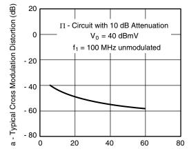
$_{95\,9733}$   $\,$   $f_{2}$  , modulated with 200 kHz, m = 100 % (MHz) Fig. 3 - Typ. Cross Modulation Distortion vs. Frequency  $f_{2}$
