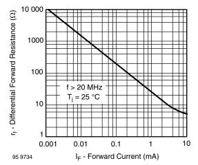
Fig. 2 - Differential Forward Resistance vs. Forward Current
