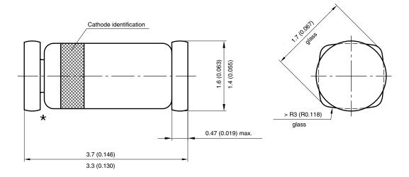
★ The gap between plug and glass can be either on cathode or anode side
