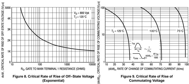
Figure 8. Critical Rate of Rise of Off-State Voltage (Exponential)
