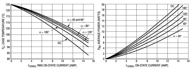
Figure 1. RMS Current Derating
