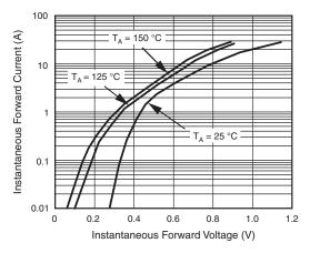
Fig. 3 - Typical Instantaneous Forward Characteristics
