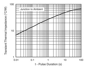
Fig. 6 - Typical Transient Thermal Impedance
