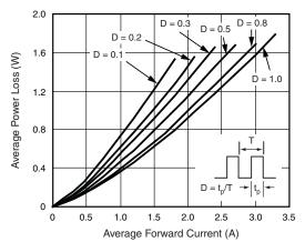
Fig. 2 - Forward Power Loss Characteristics
