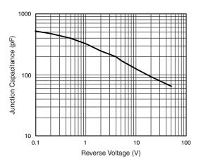
Fig. 5 - Typical Junction Capacitance
