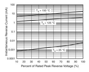
Fig. 4 - Typical Reverse Characteristics
