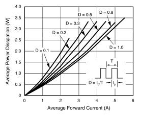
Fig. 2 - Forward Power Dissipation Characteristics
