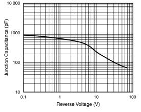
Fig. 6 - Typical Junction Capacitance
