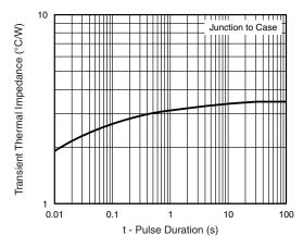
Fig. 5 - Typical Transient Thermal Impedance
