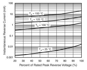
Fig. 4 - Typical Reverse Characteristics
