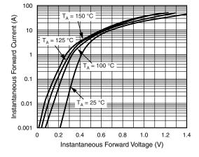
Fig. 3 - Typical Instantaneous Forward Characteristics
