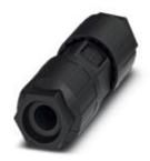
QUICKON cable connector, black, 4+PE-pos., 2.5 mm<sup>2</sup> ... 6.0 mm<sup>2</sup>/690 V/40 A, for cable diameter of 9 mm ... 14 mm
