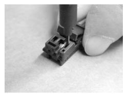
Insert Tool Into Second Window and Pull Wire
