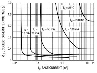
Figure 3. Collector Saturation Region
