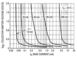
Figure 9. Collector Saturation Region
