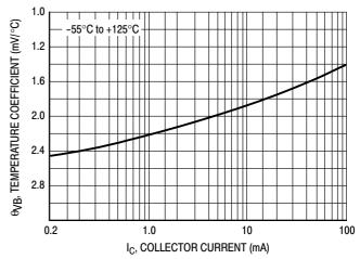
Figure 4. Base-Emitter Temperature Coefficient
