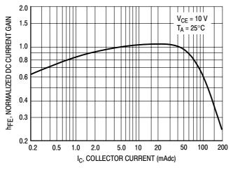
Figure 1. Normalized DC Current Gain
