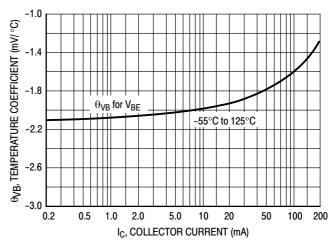
Figure 10. Base-Emitter Temperature Coefficient
