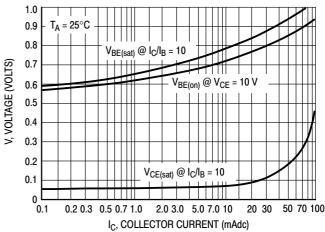
Figure 2. "Saturation" and "On" Voltages
