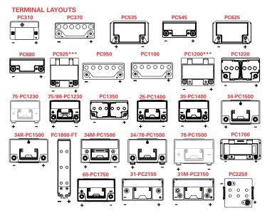
Drawing sizes are for terminal position reference only; diagrams are not proportionate to each other. \*\*\*Optional Reversed Polarity (L)
