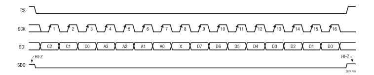
Figure 10. SPI Interface Timing (Write or WrtUpd)
