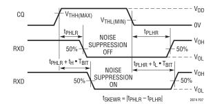
Figure 7. Receiver Timing
