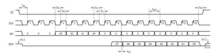
Figure 9. SPI Interface Timing (Read)
