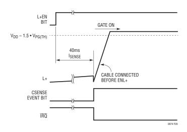
Figure 20. Cable Sense Behavior: Connection Before ENL+
