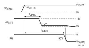
Figure 1. L+ Pin Overcurrent
