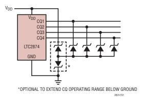
Figure 31. TVS Diode Protection for CQ pins
