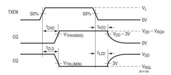
Figure 6. Driver Enable/Disable Timing
