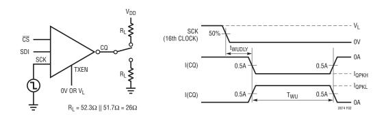
Figure 2. Wake-Up Parameters
