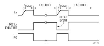
Figure 25. Latchoff Fault Behavior (for L+ Short)
