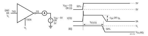
Figure 3. CQ Pin Overcurrent
