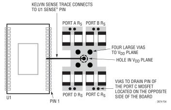
Figure 34. Good PCB Layout Example
