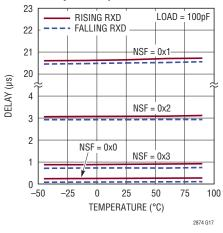
Receiver Pulse Rejection and **Detection Delay vs Temperature**
