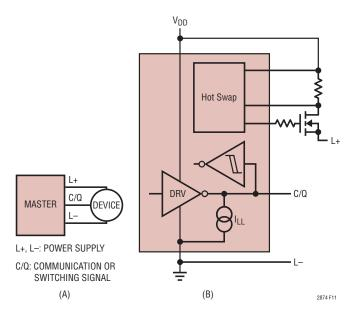
Figure 11. (A) SDCI Class A 3-Wire Interface (B) LTC2874 Master 3-Wire Interface Port
