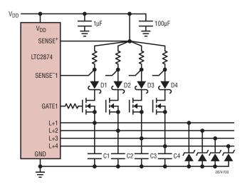
Figure 30. Reverse Protection and TVS Diode Protection for L+ Outputs
