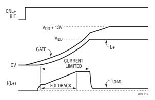
Figure 16. L+ Enable Behavior with Foldback
