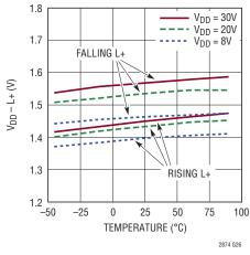
Logic Input Threshold vs **V<sub>L</sub> Supply Voltage**
