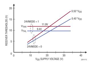
Figure 12. CQ Receiver Input Threshold (Typical)
