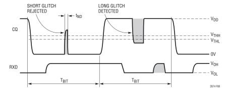
Figure 8. Receiver Noise Suppression
