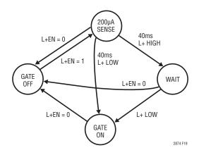
Figure 19. Cable Sensing State Diagram
