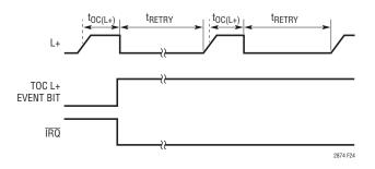
Figure 24. Auto-Retry Fault Behavior (for L+ Short)
