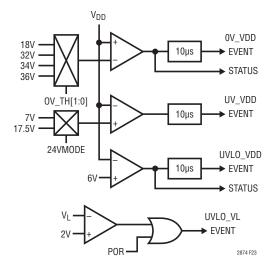
Figure 23. Supply UVLO, UV, and OV Monitors
