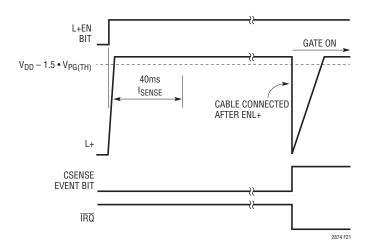
Figure 21. Cable Sense Behavior: Connection After ENL+
