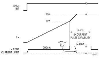
Figure 17. L+ Current Pulse Capability
