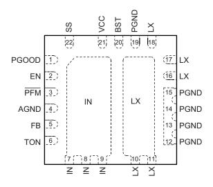
22-Pin 4mm x 4mm QFN (Top View)
