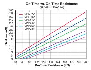
Figure 3.  $T_{ON}$  vs.  $R_{TON}$  Curves for AOZ2261QI-15
