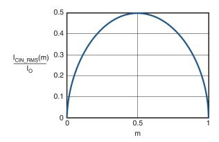
Figure 4. I<sub>CIN</sub> vs. Voltage Conversion Ratio
