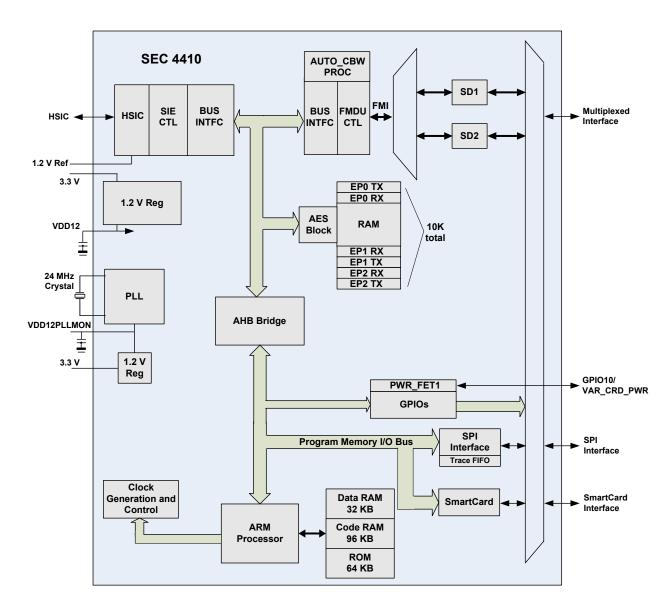
Figure 2 SEC4410 Block Diagram
