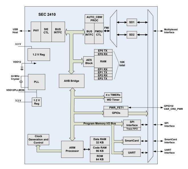
Figure 1 SEC2410 Block Diagram
