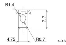
Solder Terminal (It can be used for TAB #187)
