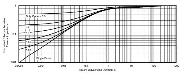
Normalized Thermal Transient Impedance, Junction-to-Ambient
