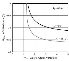
On-Resistance vs. Gate-to-Source Voltage
