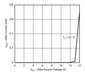
Gate Current vs. Gate-Source Voltage
