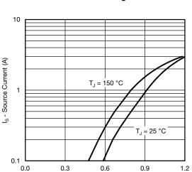
$V_{\text{SD}}$  - Source-to-Drain Voltage (V) Soure-Drain Diode Forward Voltage
