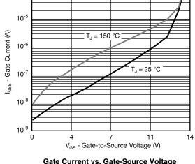
Gate Current vs. Gate-Source Voltage
