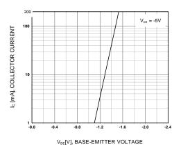
Figure 3. Base-Emitter On Voltage
