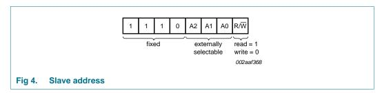
The read/write bit must be set LOW to enable a write to the Control register, or HIGH to read from the Control register.
