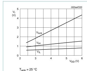
Fig 9. Typical input levels versus supply voltage
