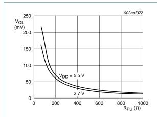
Fig 11. Typical LOW-level output voltage versus pull-up resistance
