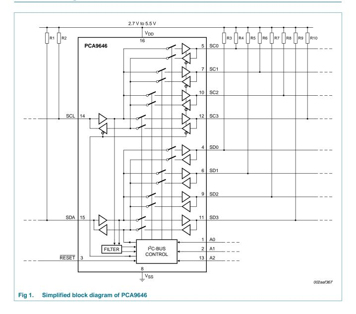
**Buffered 4-channel 2-wire bus switch**
