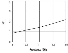
**Insertion Loss vs. Frequency**
