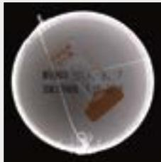
The seal and engraved text affect the image, and the shrink seal cannot be sufficiently detected.
