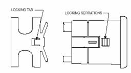
LOCKING TAB MUST ALIGN WITH LOCKING SERRATIONS
