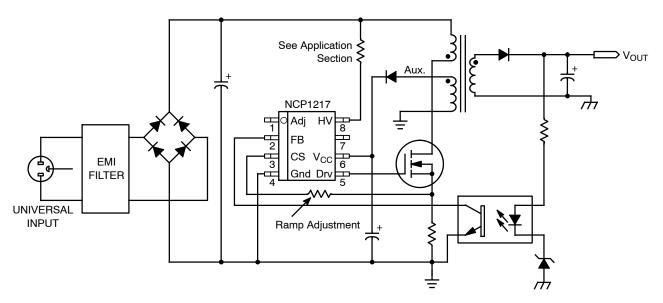
Figure 1. Typical Application Example
