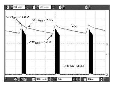
Figure 18. Typical Waveforms in Short Circuit Conditions
