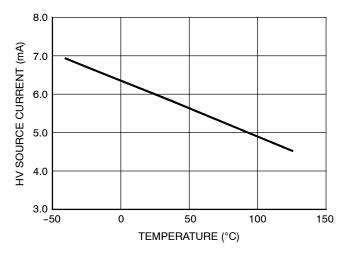
Figure 15. High Voltage Current Source (@ V<sub>CC</sub> = 10V) vs. Temperature
