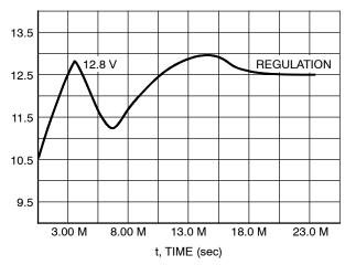
Figure 17. A Typical Startup Sequence for the NCP1217
