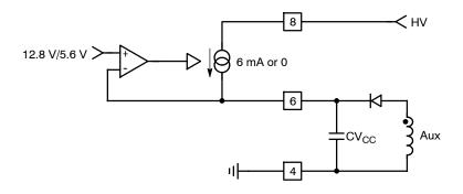
Figure 16. The Current Source Brings V<sub>CC</sub> Above 12.8 V and then Turns Off
