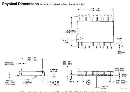
20-Lead Small Outline Integrated Circuit (SOIC), JEDEC MS-013, 0.300" Wide Body Package Number M20B
