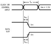
FIGURE 5. Propagation Delay, Pulse Width Waveforms
