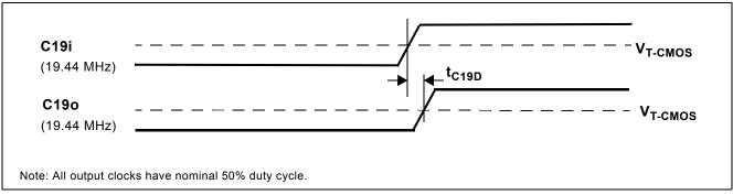
Figure 12 - C19i Input to C19o Output Timing
