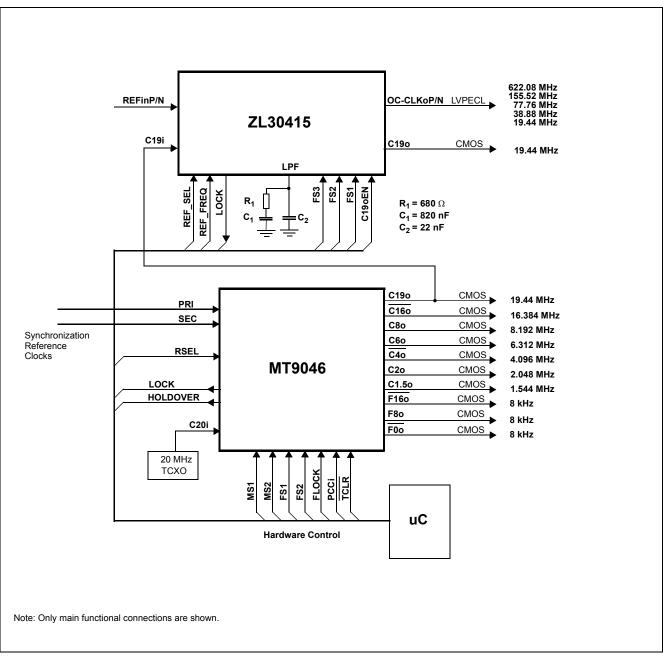
The ZL30415 in combination with the MT9046 provides an optimum solution for SONET/SDH line cards (see Figure 6).
