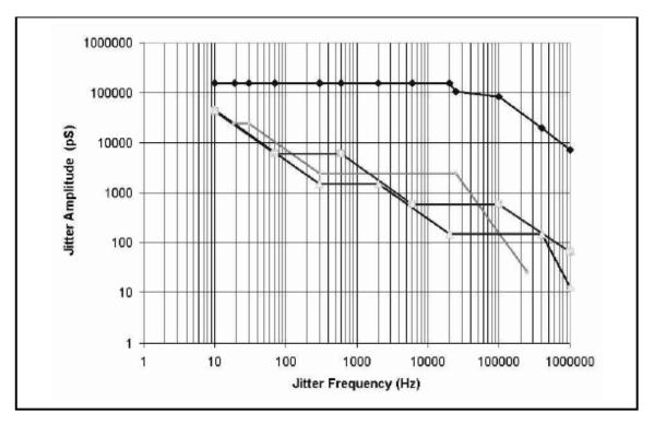
Figure 4 - Input Jitter Tolerance
