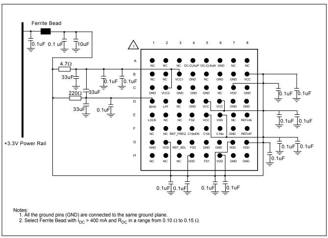
Figure 10 - Power Supply and BIAS Circuit Filtering
