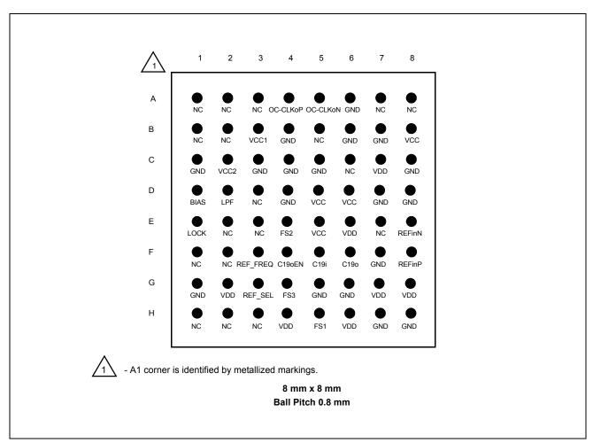
Figure 2 - BGA 64 Ball Package (Top View)
