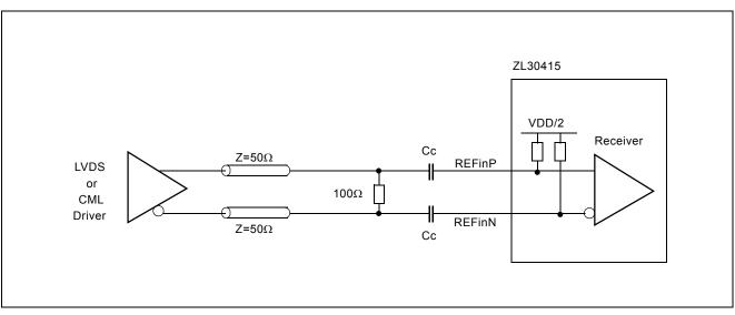
Figure 8 - Interfacing to LVDS or CML Driver
