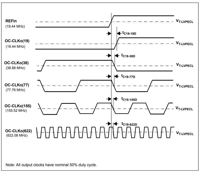
Figure 15 - REFin (19.44 MHz) Input to OC-CLKo Output Timing
