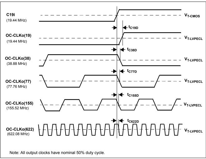
Figure 14 - C19i Input to OC-CLKo Output Timing
