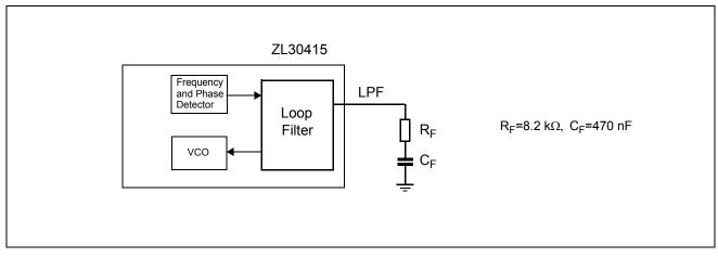
Figure 3 - Loop Filter Elements
