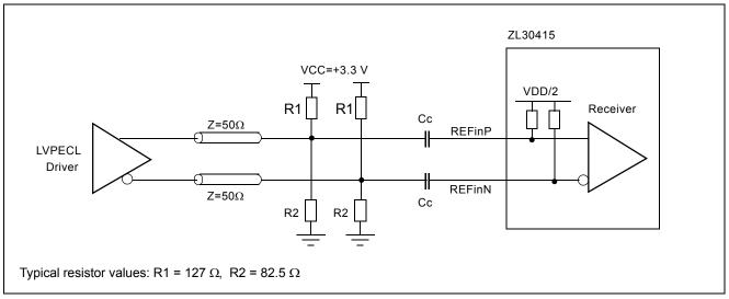
Figure 7 - Interfacing to LVPECL Driver
