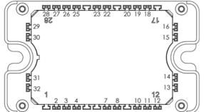
All multiple inputs and outputs must be shorted together 10/11/12; 7/8; 27/28; ...
