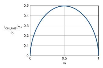
Figure 2. I<sub>CIN</sub> vs. Voltage Conversion Ratio
