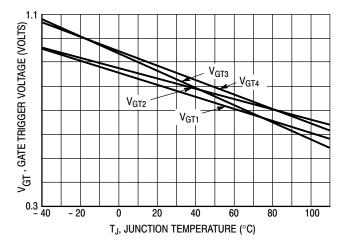
Figure 16. Gate Trigger Voltage Variation
