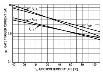
Figure 14. Typical Gate Trigger Current Variation
