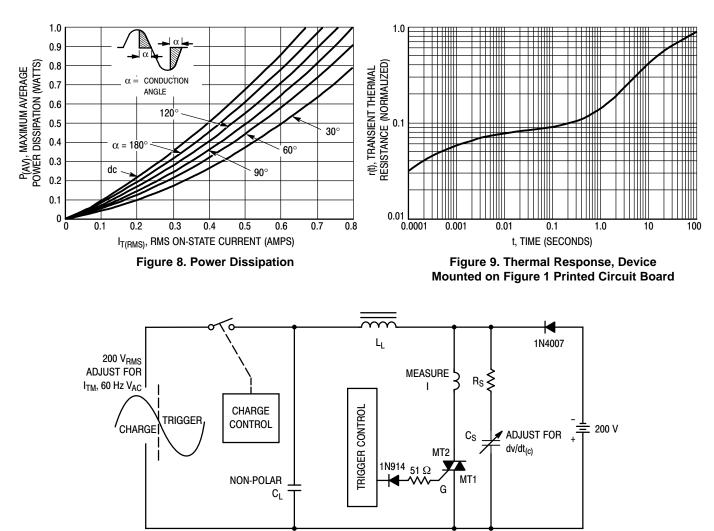
Note: Component values are for verification of rated (dv/dt)<sub>c</sub>. See AN1048 for additional information.
