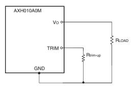
Figure 21. Circuit Configuration to trim-up output voltage.
