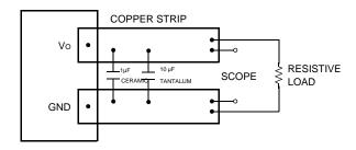
Note: Scope measurements should be made using a BNC socket, with a 10  $\mu$ F tantalum capacitor and a 1  $\mu$ F ceramic capcitor. Position the load between 51 mm and 76 mm (2 in and 3 in) from the module
