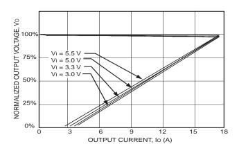
Figure 2. Output Voltage and current characteristics.
