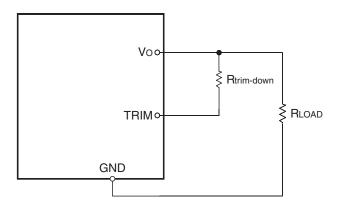
Figure 22. Circuit Configuration to Decrease Output Voltage.
