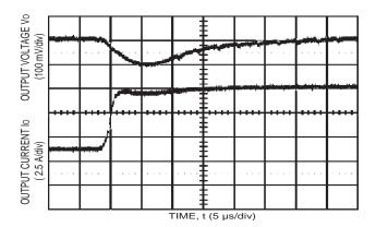
Figure 13. Typical Transient response to step load change at 2.5 A/µs from 100% to 50% of IO,max at 3.3 V Input (Cout =1 µF ceramic, 10 µF Tantalum).
