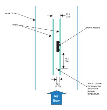
Figure 25. Thermal Test Setup.
