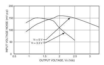
Figure 18. Input Voltage Ripple for Various Output Models, IO = 10 A (CIN = 150  $\mu$ F polymer // 47  $\mu$ F ceramic).
