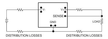
Figure 23. Effective Circuit Configuration for Remote Sense Operation.
