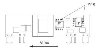
Figure 24. Temperature Measurement Location.
