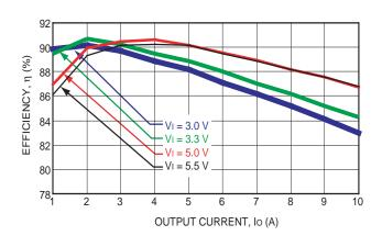
Figure 5. Converter Efficiency vs Output Current AXH010A0P (1.2V Output Voltage).
