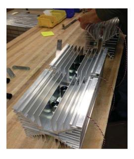
Fig. 8 - Step 6: Check to make sure the two mounting surfaces are still parallel. Tighten each bolt a 1/10<sup>th</sup> turn more.
