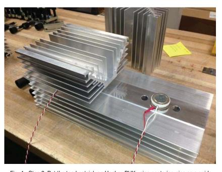
Fig. 4 - Step 2: Put the top heatsink on Hockey PUK using centering pins as a guide, and rotate the heatsink back and forth to distribute the paste evenly.
