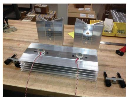
Fig. 3 - Step 1: Clean the surface of the heatsink then put thermal paste on the Hockey PUKs.
