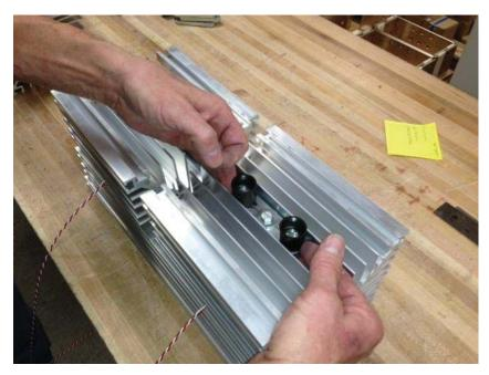
Fig. 5 - Step 3: Drop the clamp into the top heatsink
