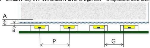
**Common Terms Graphic.** Uniformity tape allows greater G distance, thus improving the A/P ratio. In addition, by increasing the freedom for the G gap, shorter LEDs can be used, thus potentially reducing material cost of LED part.
