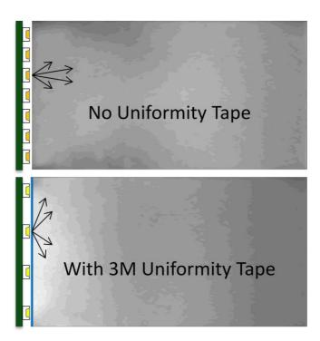
**Light distribution comparison.** Images above show a light guide optimized for a backlight without Uniformity Tape. When Uniformity Tape is applied, the brightness intensity increases near the light source, and drops further away, which requires an extraction pattern adjustment.
