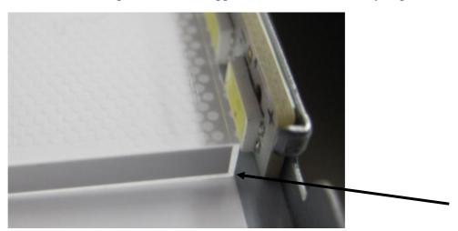
**Edge Reflector.** An Edge reflector should be used on all non-illuminated edges of the light guide with Uniformity Tape. In order to prevent loss of brightness, edges closest to the light source are most critical to cover with a reflector.
