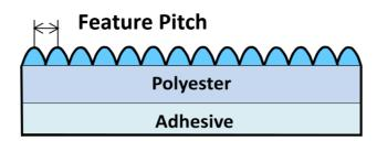
Polyester film thickness: 50 μm Adhesive thickness: 50 μm Feature pitch: 24 μm
