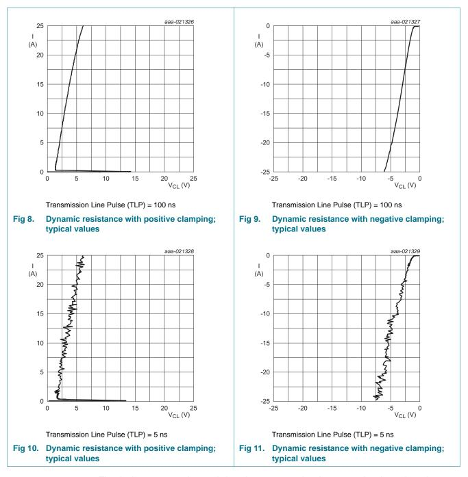
The device uses an advanced clamping structure showing a negative dynamic resistance. This snap-back behavior strongly reduces the clamping voltage to the system behind the ESD protection during an ESD event. Do not connect unlimited DC current sources to the data lines to avoid keeping the ESD protection device in snap-back state after exceeding breakdown voltage (due to an ESD pulse for instance).
