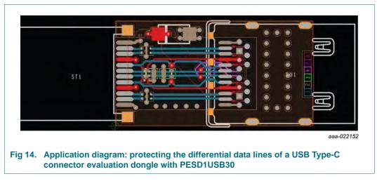
Since the SuperSpeed TX/RX lines are separated by GND or VBUS from the Hi-Speed lines, PESD1USB30 makes it easy to achieve same signal lengths, straight routing, and optimal positioning for ESD protection directly at the connector.
