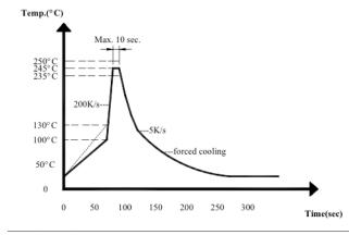
Recommendable wave soldering condition is as follows:
