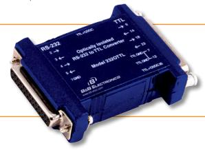
Models 232TTL and 2320TTL convert RS-232 signals to 0-5 VDC TTL levels. The 2320TTL provides 1500V optical isolation. Two channels are used to convert from RS-232 to TTL signals and two channels are used to convert fomr TTL signals to RS-232.
