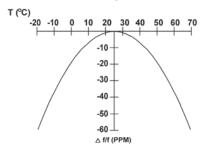
To determine frequency stability, use parabolic curvature (K). For example: What is stability at 45  $^{\circ}\!\!C?$
