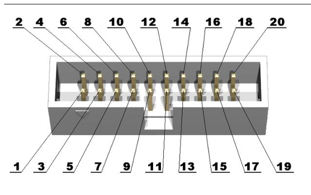
**TMS** Input **Test Mode Select.** The TMS pin selects the next state in the TAP state machine.
