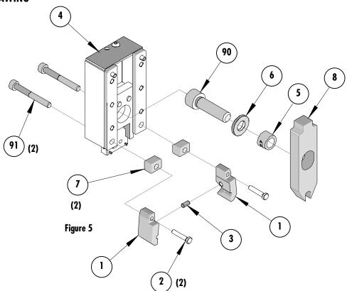
Note: The bushing (item 5) is included with the Funnel Slide Assembly; however, it is not necessary for installation on the molded strip applicators.
